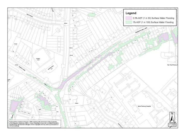
Figure 2 – Surface water flood risk within the Yew Tree Lane, Cornyx Lane and Wherretts Well Lane Area, Silhill.
