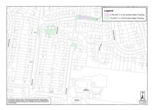
Figure 5 - Surface water flood map within the Coppice Road area, Elmdon
