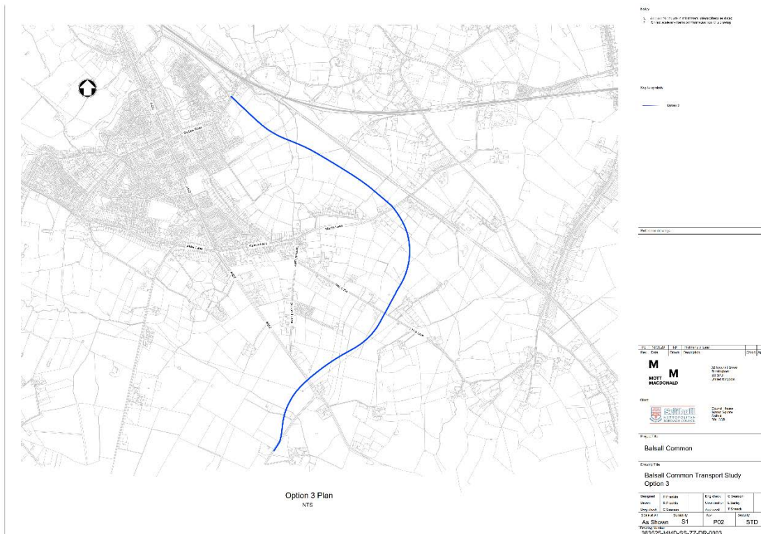
Figure 8.4: Alignment 1 Dual carriageway (50mph)
