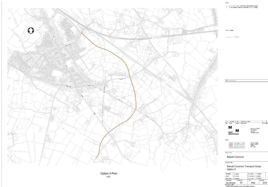
Figure 8.6: Alignment 2 Single carriageway (50mph)
