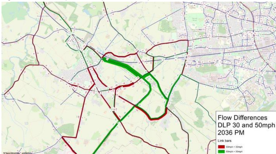
Figure C.2: DLP 30mph and 50mph Link road Options 2036 PM
